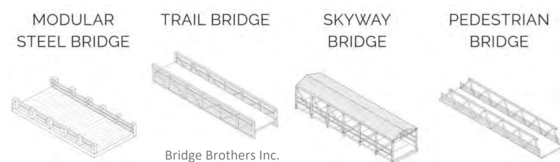
FIGURE 4: ALTERNATE PED BRIDGE CONFIGURATIONS
